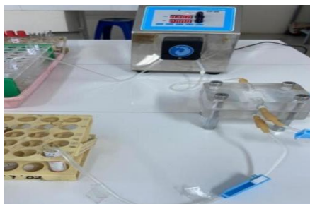
Gambar 1. Prototype alat hemodialisa
